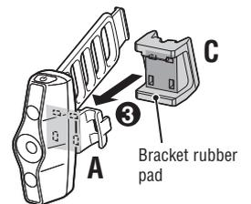
Attach the bracket rubber pad (C) aligning it with the protrusion on the back of the bracket (A).
