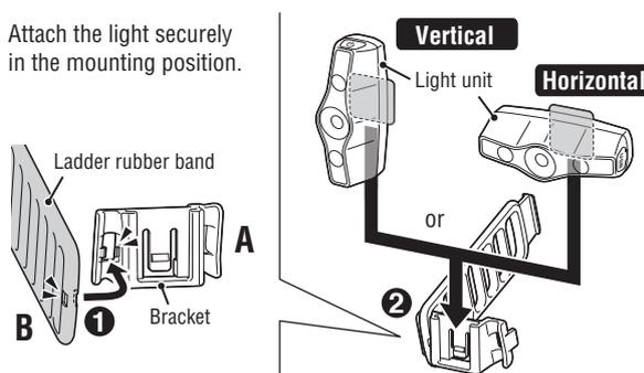
Attach the ladder rubber band (B) to the bracket (A).
